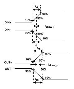
FIGURE 6A. MEASUREMENT POINTS
